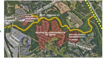
The recommended alternative alignment of Segment 11 runs along the original alignment but stops at Kempsford Drive and adds intersection improvements at Harris Houston Road and Kempsford Drive. The recommended alternative balances safety, costs, community priorities, long-term maintenance, and proximity of amenities and connects 605 dwellings including Pavilion Apartments (150), Houston Hills Neighborhood (385), and Hunting Ridge Neighborhood (70).
