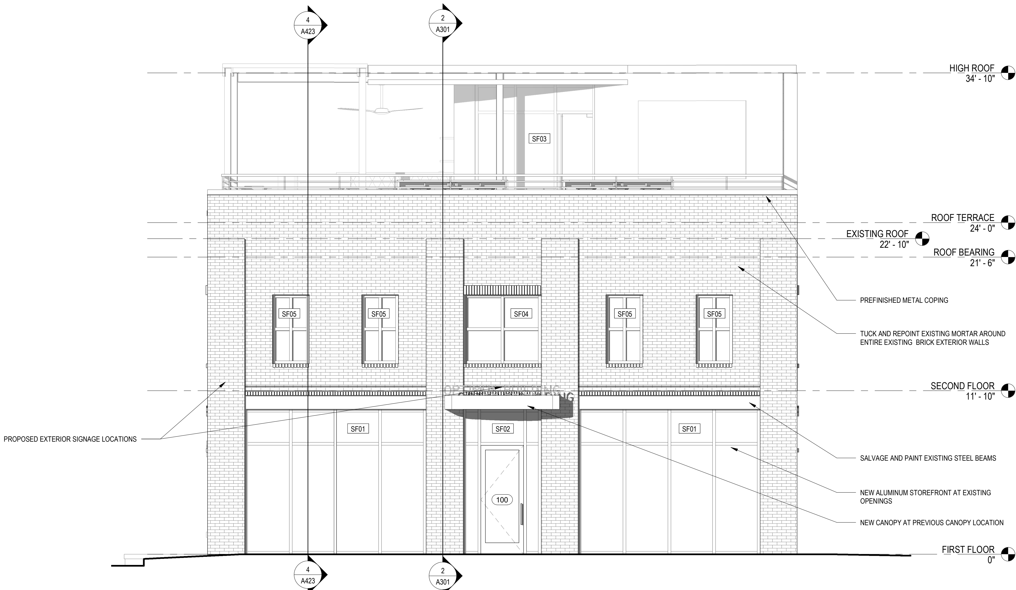
SOUTH ELEVATION SCALE: 1/4" = 1'-0" R.E. = 1/A101
