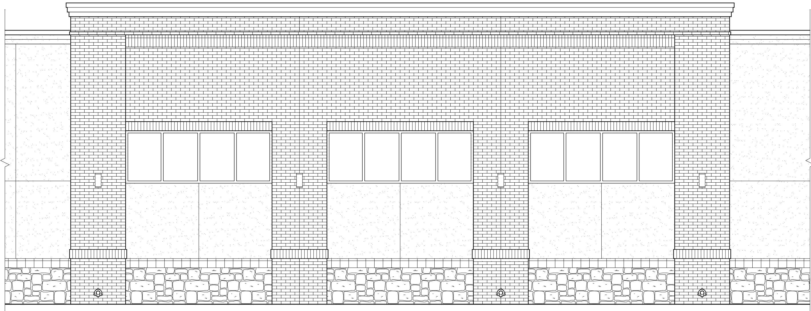
04 ENLARGED ELEVATION: Left Side Facing South 1/4" = 1'-0"
