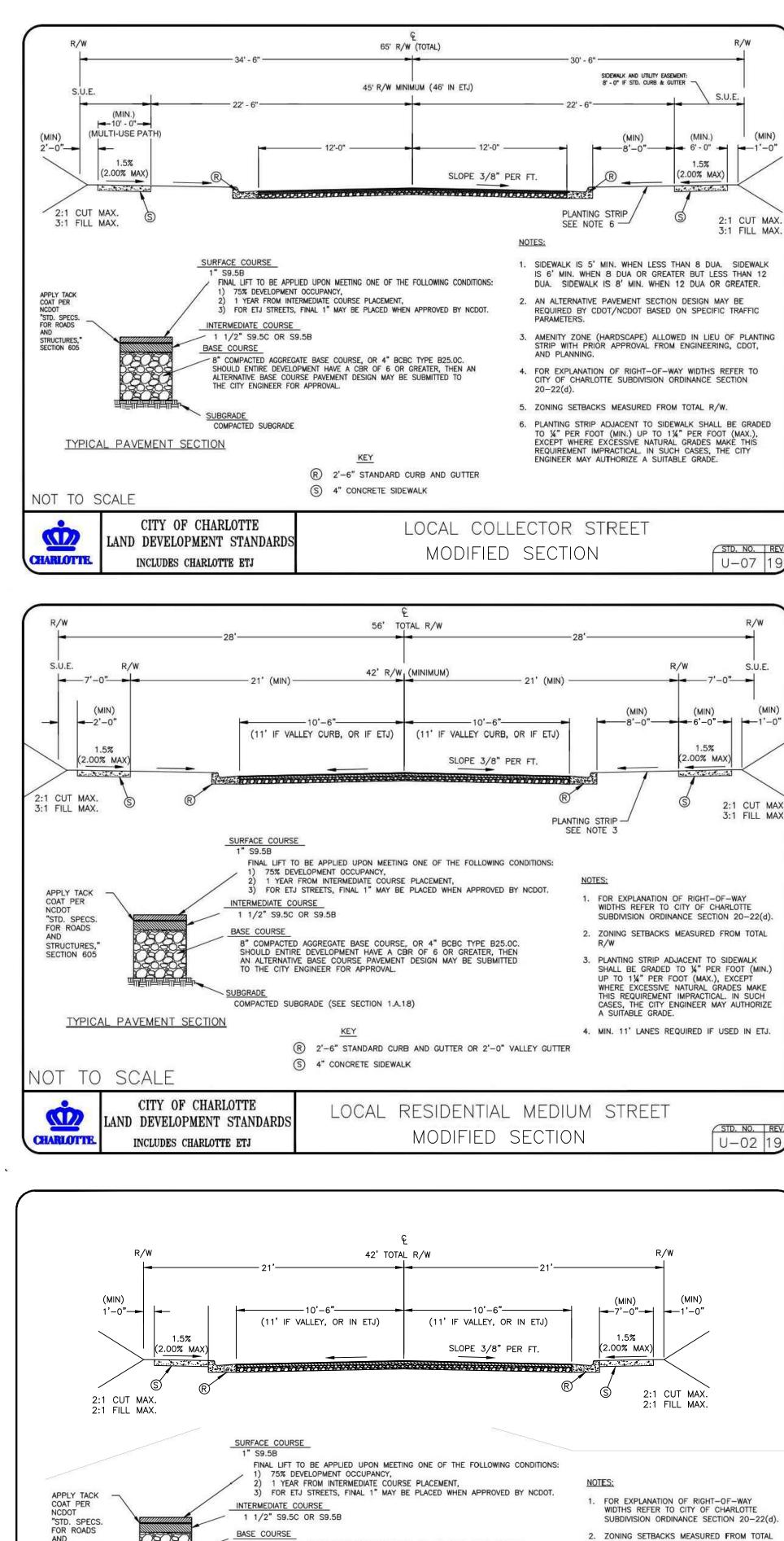
BASE COURSE B" COMPACTED AGGREGATE BASE COURSE, OR 4" BCBC TYPE B25.0C SHOULD ENTIRE DEVELOPMENT HAVE A CBR OF 6 OR GREATER, THEN AN ALTERNATIVE BASE COURSE PAVEMENT DESIGN MAY BE SUBMITTED TO THE CITY ENGINEER FOR APPROVAL. SUBGRADE
