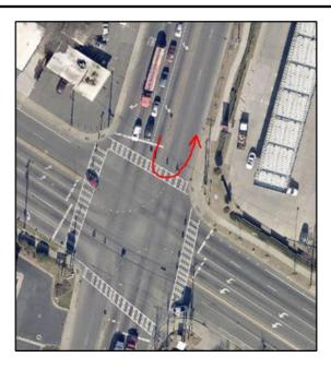
3.—Petitioner to evaluate the construction of a directional crossover for left turn movements into the site at the proposed access on N Sharon Amity Rd by providing site plan exhibit(s) to evaluate protentional impacts and determine feasibility.
