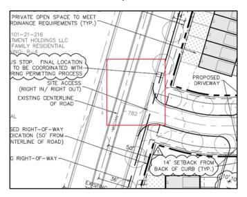
4.—The site is located along CATS local bus route #29 and #229 on N. Sharon Amity Road. CATS requests the construction of an ADA compliant bus amenity on N. Sharon Amity Road with a bus shelter pad at the northern edge of the development for existing bus routes, CATS detail 60.05A The final location and type of amenity will be coordinated with the developer through the permitting process. Addressed
