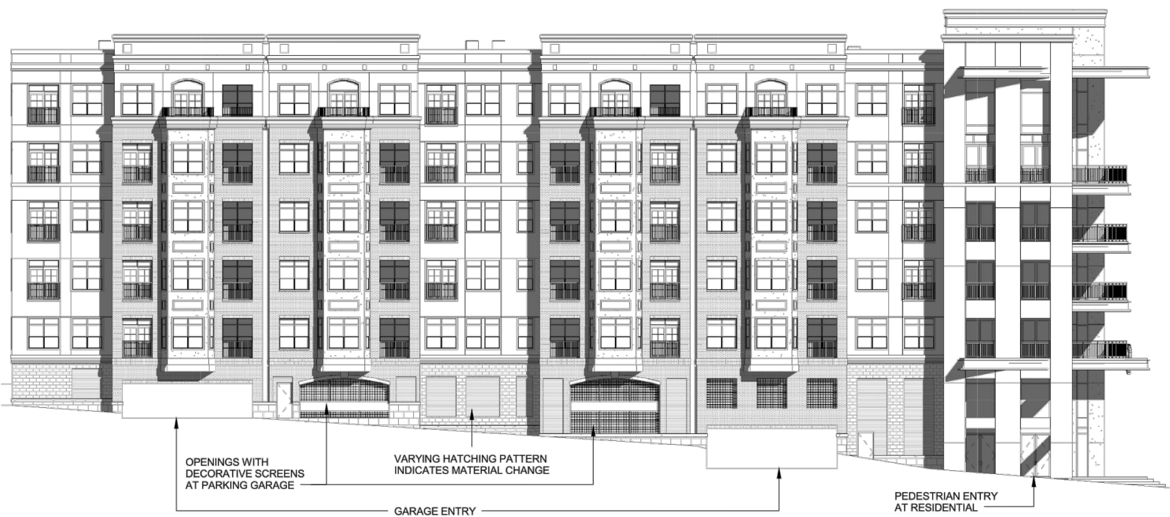
C HARDING PLACE ELEVATION / SECTION SCALE: 1"=20' - 0"
