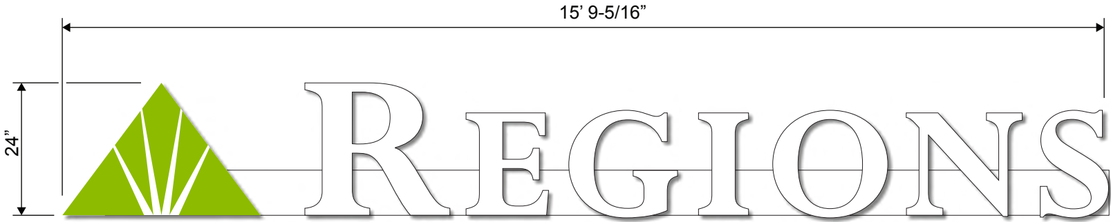
RFC.REG-IL24MWL-RW - 24”H ILLUMINATED WHITE MODIFIED LINEAR RACEWAY CHANNEL LETTERS SCALE: 1/2” = 1’ 0”
