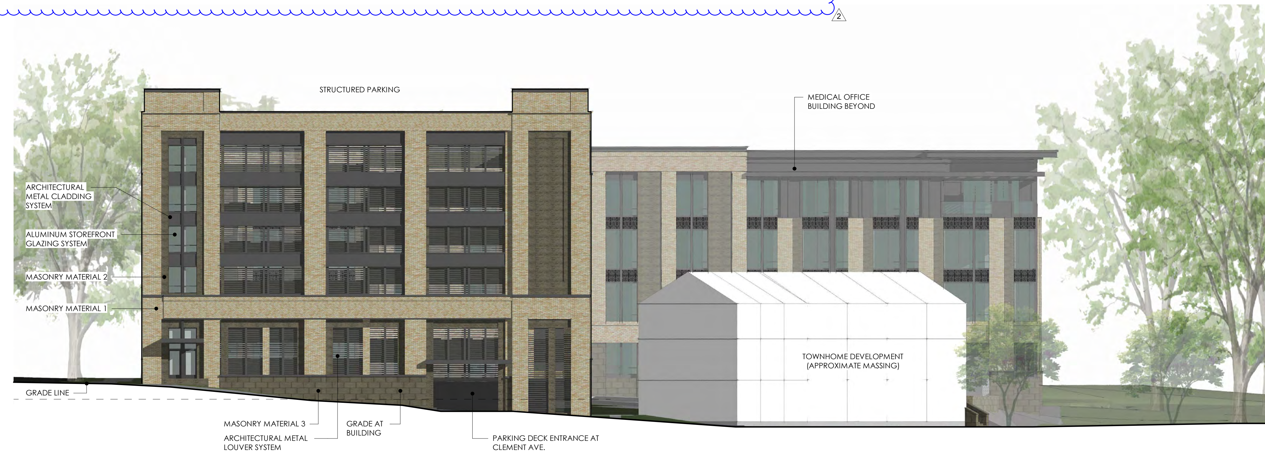
2 RZ-05 CLEMENT AVENUE ELEVATION SCALE: 1/16" = 1'-0"
