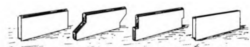
Above: Examples of concrete staves, circa 1919. 56 Below: Detail of south elevation of north silo showing its concrete stave and steel reinforcement hoop construction.
