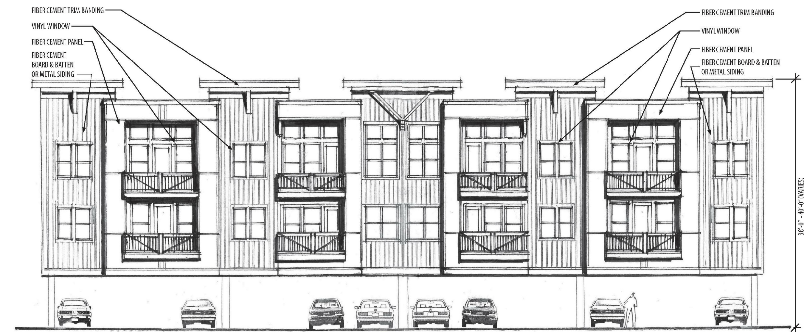
TYPICAL PARKWOOD REAR BUILDING ELEVATION
