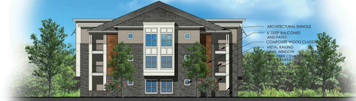
3 Story Garden Building - Side Elevation
